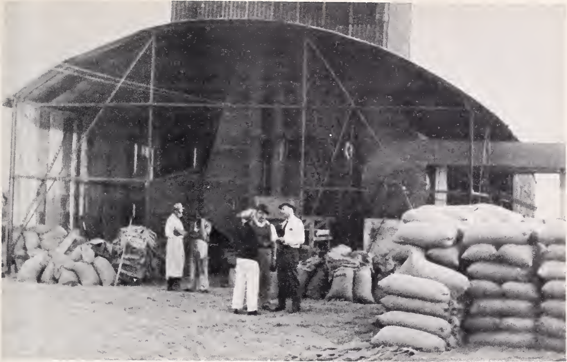
FIGURE 24. A rice dryer in Argentina. Most of the Rice of Southern Brazil and of Argentina is dried in on-farm rice dryers, which use wood for fuel.
